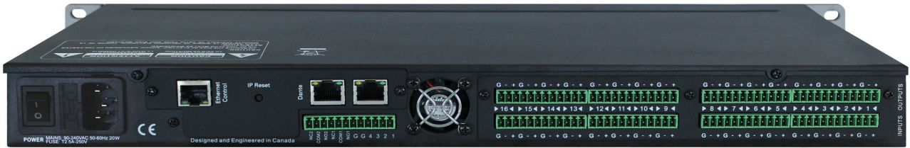
Rear panel view of the Neutrino A1616-N Dante-enabled DSP.
