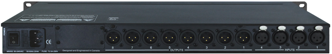
Above: Rear panel view of the XA4080, with XLR I/O section.
