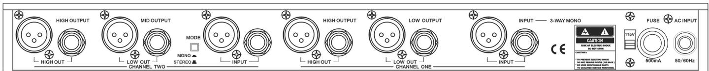
It is easy to interface the unit with a wide variety of equipment. The rear panel has balanced XLR and 1/4" phone jack connectors.
